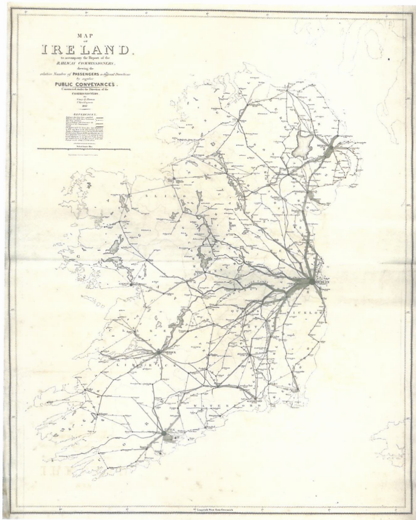
The Royal engineer Lieutenant Henry Drury Harness drew this map in 1837 as part of an atlas to accompany a report by the Irish Railway Commissioners. It is considered to be the first flow map and preceded Minard's work by a few years. However, there is no sign that the latter had any knowledge of this atlas.
