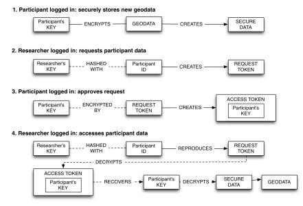
Fig. 5. OpenPaths security model, © 2012 The New York Times Company
